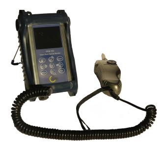
Oxin Optical Fiber Microscope, OFM-100, is used to inspect end-face of fibers and check the optic connectivity. It magnifies fibers of 125um diameter 200-400 times, enlarging picture through a video signal to the display where the status of fiber end-face is showed clearly in the end.
